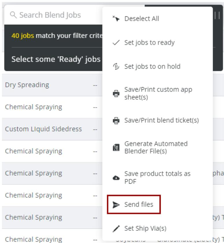
8. Browse to the desired files to be sent to the applicator and select **Send**. The applicator should receive the files on the Raven monitor.
