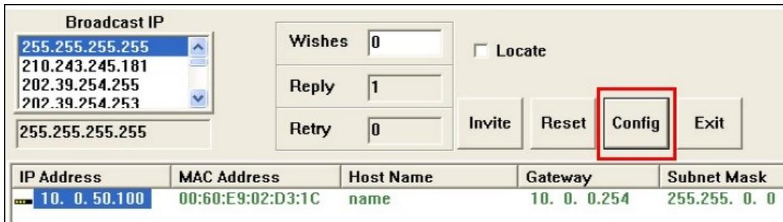
Edit the information on the *Dialog* window, and designate fields as desired to match the domain's network. Set up a static IP address.
