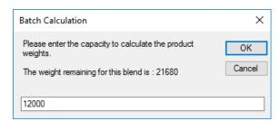
After the Capacity has been entered, choose the Get Blend Time button on the Ranco Interface tab. Start mixing product by choosing the following buttons from left to right: I/U Start, Elevator Start, Blend Start, and Meter Start.
